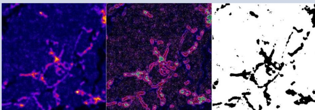
Original CARS image, (b) – Sobel-Feldman operator image processing, (c)– separated pixels of DNA on graphene-covered glass
