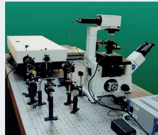
A home-built CARS microscope (Center for Physical Sciences and Technology, Vilnius, Lithuania) with a simple and compact laser (EKSPILA Ltd.) was used. The cell images are registered in the forward and EPI mode at the 1600, 1360 and 2800 cm<sup>-1</sup> region.
